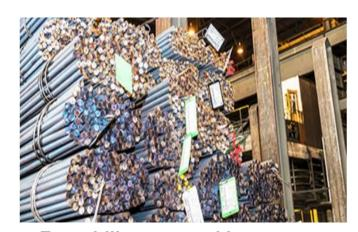
► From billets to steel bars (~32% of sales) Bundle weight 4–6 tons/ 16–66 mm (round)/ 17.7–62 mm (hexagonal)/ 16–40 mm (ribbed)
